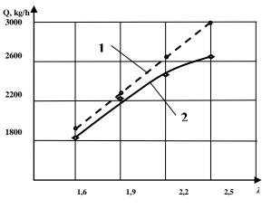
Figure 3: Dependence of capacity Q of the kinematic mode  $\lambda$ . (1- calculated Q = f ( $\lambda$ ), 2 - actual)
