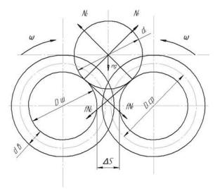
Figure 1: Schematic of the interaction with the screw root c
